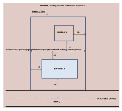
Limiting distance determines the number of glazed openings permitted in an exposing building face (Table 9.10.15.4.) and determines other construction requirements such as protection of soffits and fire resistance rating of cladding. When limiting distance is less than 1.2 meters, glazed openings are not permitted in the exposing building face.
